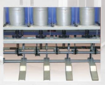
A highly efficient foot-operated braking system provides easy stopping of the spindle. The braking system disengages the tegential belt from the spindle resulting in longer life of the belt.
